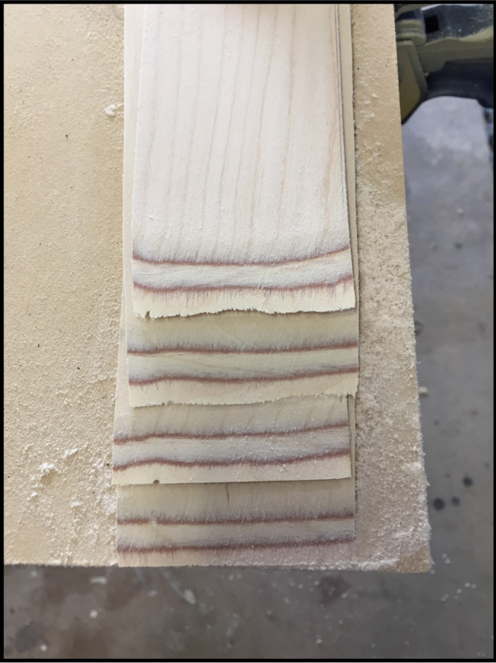
Scarf joints on 1.5 mm spar skins
