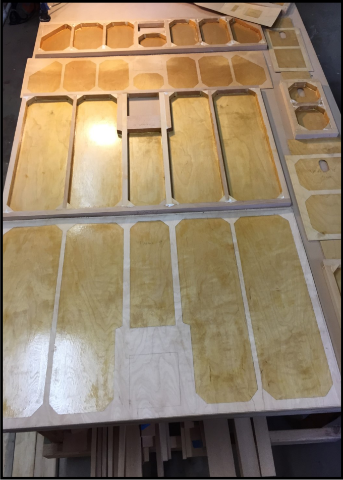
Two coats of varnish on frames and skins. (Note bare wood areas where glue will be applied)
