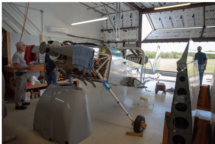
Stevens RV-14 has the engine hung and is getting its complement of avionics
