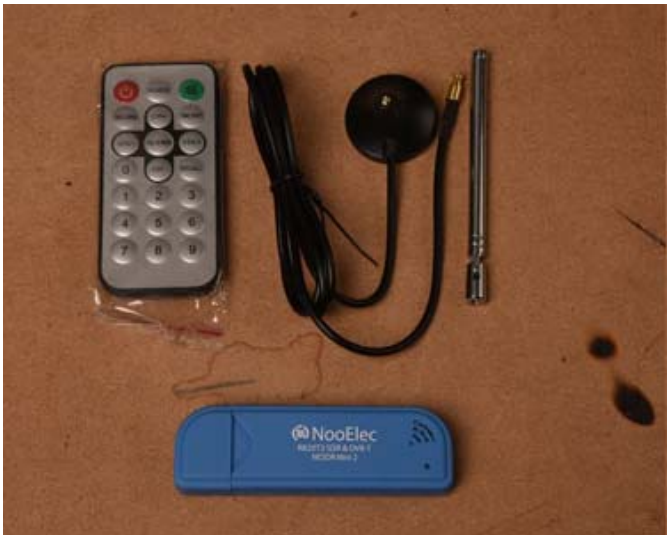
The NESDR 2 comes with a telescopic antenna and a remote control (the latter not needed for this project)
