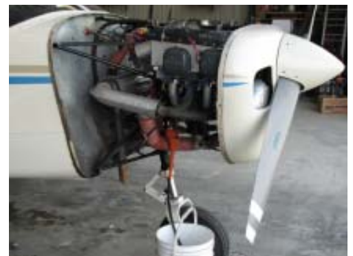
Set up for a clean oil drainage
