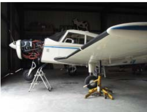
All jacked up ready to clean and pack the wheel bearings
