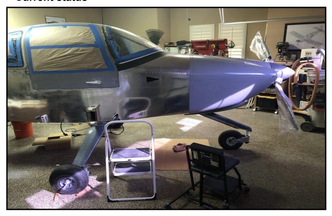
Engine in (Aerosport built IO-540)
