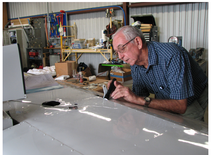
Steve Sewell checks location of the mounting nuts for the vertical stabilizer
