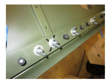
My next attempt at stopping the carnage is to place a bolt in the hole that should not receive a rivet.
