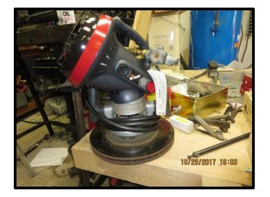
I once got caught at Oshkosh during the summer when the temperature at night dropped into the thirties. I vowed not to make that mistake again. I came up with this contraption. It is a Mr. Heater affixed to a router base – bolted to a brake rotor. I have discovered that if you use a wood router to cut aluminum, it tends to destroy the router. When this happens, you cn convert the router into a heater. I thought it would be completely safe in our tent.
