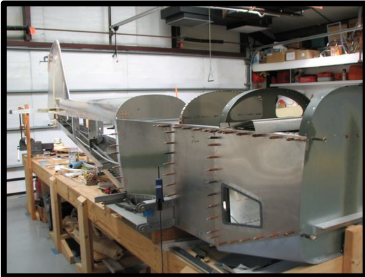
The fuselage now straightened and getting the control system installed
