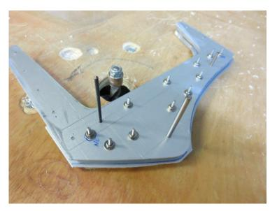
This is where all of the work pays off. I use the part I have been working on as a template. The router table has a ball bearing edge trimmer bit for making duplicate parts at little to no effort.
