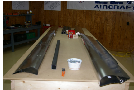
Fabrication of the Slats
