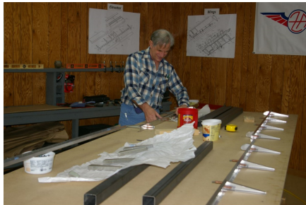
Fabrication of the Flaperons
