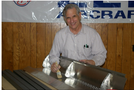
Fabrication of the Slats
