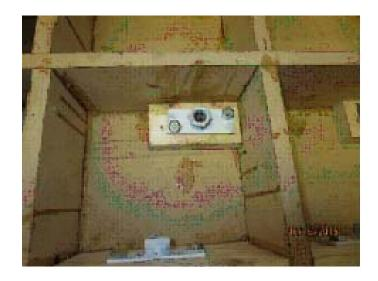
My son welded hundreds of these nut plates up. All of the work I have described so far was to build a 4x10 table. I need a 4x18 foot table. The two tables have to be seamed up using these internal nut plates.
