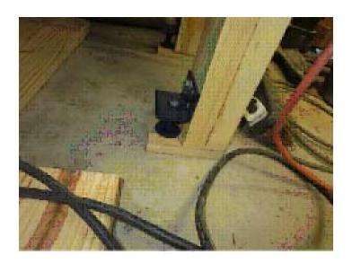
My garage floor has as serious slant. Each leg has its own adjustment for level.
