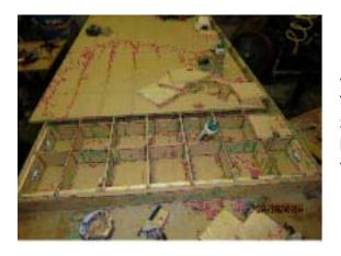
I then took another sheet of 1/2 mdf and cut many uniform width slices. Did I mention how important my table saw was? Then I slowly made a grid using wood glue. I must have spent \$40 on glue. The waxed table will not let the glue adhere. My belief was that the grid would have to follow the flat contour of the waxed table.
