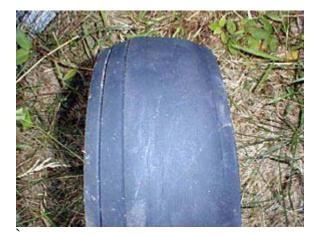
This tire suffered from both overinfaltion and alignment problem. Aircraft with tire wear problems, not attributable to tire balance, ned to have the alignment checked. Check your maintenance manual for applicability and specific procedures. Some aircraft have very limited adjustments. Inflation should also reflect the load and temperature profile on heavier aircraft.
