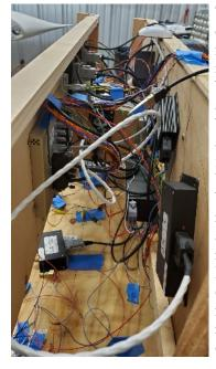
This was a great help in determining where all the remote boxes will mount, mostly on the middle bulkhead. There are almost as many boxes behind the panel as there are in the panel. This includes Vertical Power VP-X, two backup batteries, Dynon com radio, two ARINC-429 adapters, ADS-B receiver, Engine Monitoring System (EMS), SkyView network hub, and nav/strobe light controller. The Dynon ADAHRS and pitch
