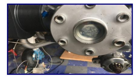
Removing the oil line is easy and capping the fittings is trivial.
