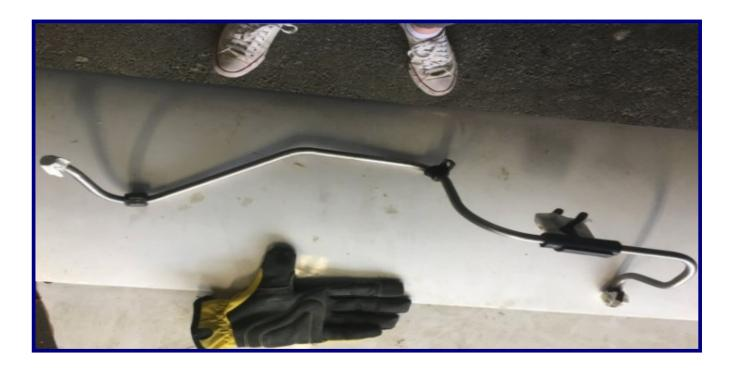
Removing the oil line is easy and capping the fittings is trivial.
