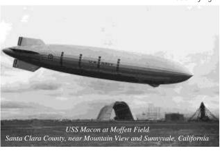
was a German idea improved upon and completed in the form of the USS Macon. A mechanical arm, referred to as a trapeze, would lower down out of the hangar bay to pick up approaching trapeze-bar equipped aircraft. Five scout planes could be snatched or launched from the Macon. The Macon was powered by 8 twelve cylinder engines.
