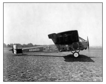
Having performed its notable feat, the big craft now rests in the Aircraft Building of the Smithsonian Institution in Washington. Its wingspread is 74 feet 10 inches; its length, 49 feet; and its height, 11 feet. The power-plant is a 400 H.P. Liberty engine. The old map of the United States showing the route followed by Macready and Kelly is still pasted in the fuselage.
