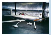
This is my project. It is a Silhouette. FAA signed it off in mid July (04). Power is via dual carbed Rotax 447. Wingspan is 32'. Cruise is to be ~125 mph. It is hangared at Stevens Point. I am currently in the test phase. It has done a low pass over runway 21/03 at STE. I started the project in '93. After many starts and stops, it's finally finished.
