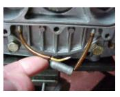
The oil injection system had been removed and the oil lines had been plugged with a wire! These must be air tight! The bottom end of a two stroke engine must not have any air leaks or the fuel air ratio will not be correct, an air leak here will eventually lead to an engine seizure. If you look at the next photo you will see an aluminum cover plate has been fabricated to cover the hole where the oil
