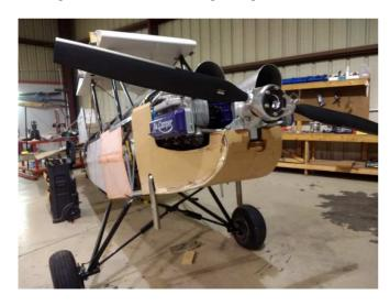
The new cowl is designed to show off Azalea's Corvair Aero-engine conversion to good effect and promises to be a head turner with new graphics and colors added.
