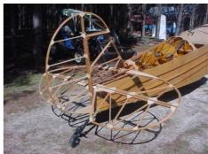
The fuel shut off and elevator trim controls were fabricated, and the cables were fitted and installed. I put the rudder, horizontal stabilizer, and elevator temporarily to check fit and to get the proper length for the elevator trim cable. Several brackets for the upper wing mount tubes have been fabricated. The lower wings and ailerons are mostly complete.
