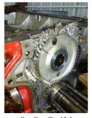
The pistons and cylinders were scavenged and installed into a new block with a new camshaft. The original heads were reinstalled. The lifters were disassembled, cleaned and returned to service. The original rods were used except for number six... An Azalea Aviation rear
