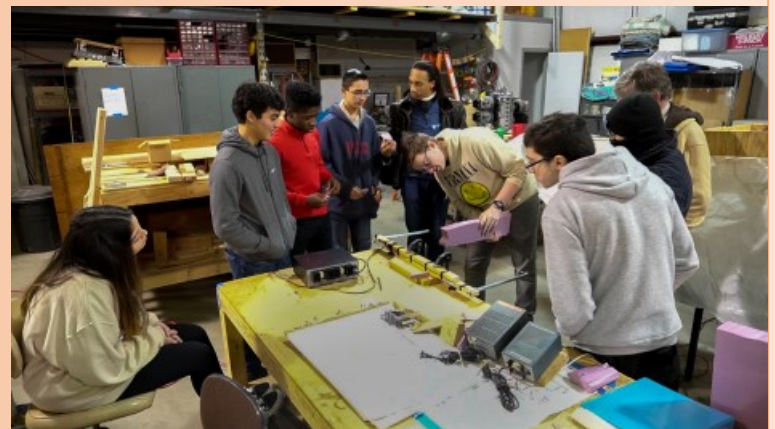
Building Youth practicing using the hot wire to cut foam for the Frankenplane horizontal stabi-
