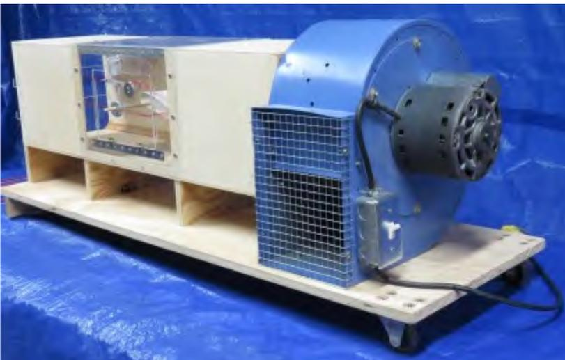
Also, with the idea of portability in mind he has rollers under the heavy blower end and a handle on the intake end so he can be rolled around much like a hand truck. Furthermore, because the blower motor end is flat and placed in the same plane as the end of the base, he can be stood up with the blower down in a stable storage position.
