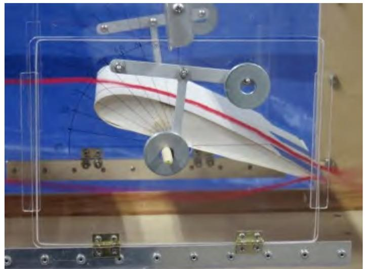
The purpose of Winston is to allow one to visualize the flow of air around a wing and get relative measures of lift and drag between different wing shapes. Learning is almost always enhanced by being able to see the issues being studied.
