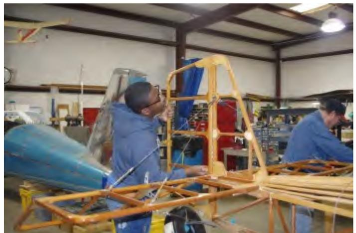
Adding the rudder for another control test
