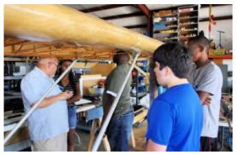
The struts are just about finished for the ultralite Piet. Next are the aileron control cables.
