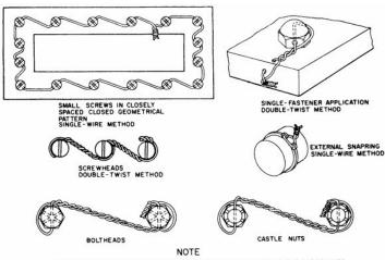
THE SAFETYWIRE IS SHOWN INSTALLED FOR RIGHT-HAND THREADS. THE SAFETYWIRE IS ROUTED IN THE OPPOSITE DIRECTION FOR LEFT-HAND THREADS.
