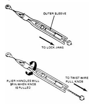
Key points to proper safety wiring:
