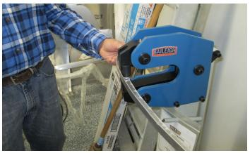
The piece of aluminum that forms the top of the exhaust tunnel was another challenging form. It starts with a straight edge at the firewall and transitions to a convex curve at the aft end. Neil made an origami-like template out of the posterboard first and you can see the fine looking result in the attached picture.
