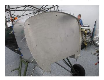
he got from his job. When he was satisfied with the fit, he then made the final part out of stainless or aluminum. The flange around the firewall is made from 5052 aluminum angle. To form that, he needed a new tool and a new skill. He purchased a Baileigh shrinker/stretcher and experimented with that on scrap until he felt ready to make the actual piece.
