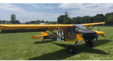
The fabric covering is made of Oratex. It's pre-painted, precolored, UV protected, and very lightweight. Covering is a one-step process: you glue it on the frame and you shrink it.
