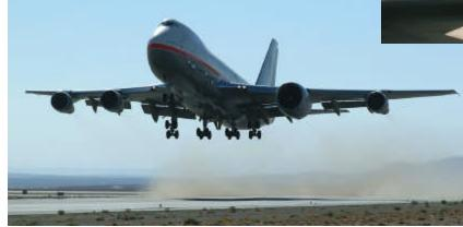
At altitude, the other three engines were throttled back and the 747 was flown at 335 knots using just the thrust generated by the GE90-115. Look at the ground clearance
