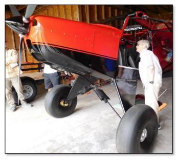
Wade's Highlander has a pair of 29-inch diameter rough terrain tires mounted on a landing gear structure that looks indestructible. The company engineer claims that you can drag the airplane, at near stall speeds, to the runway, and at an altitude of five feet, just chop the throttle and drop to the ground. With the brakes ON! That's quite a landing technique!
