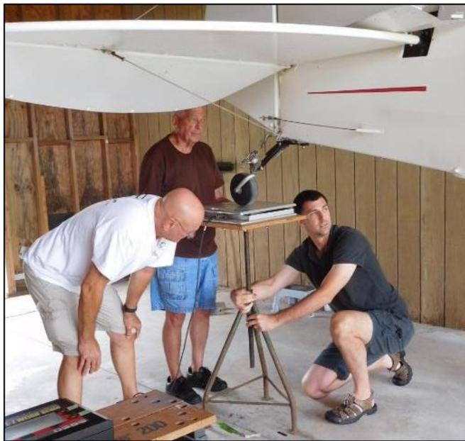
scale that rested on a welded steel stand. The stand was adjusted until the aircraft was longitudinally level. All of the fuel was drained from the tanks and then all of the engine cowlings and interior panels were rested in their proper positions.
