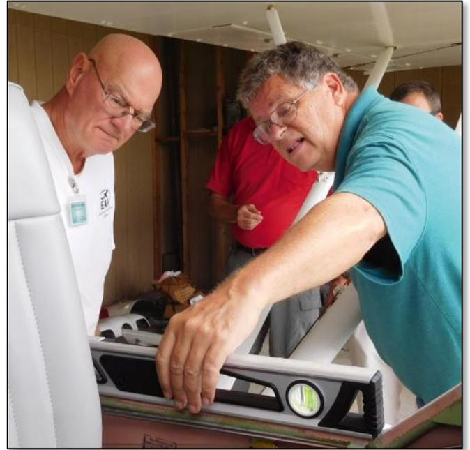
measuring the distances from there to the center of the main and tail wheels. These distances are as important as the three weights when calculating the aircraft center of gravity.
