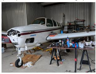
We (Pablo with a little help from me) are replacing the AI and HSI with an Aspen Avionics system. We expected this part of the project would hold up everything else except it didn't! The Aspen panel is not in the photo but its there now and has already been tested and only needs a test flight. We removed 25 pounds of gyros, back-up air pump and wires replaced with 2 pounds for the Aspen.
