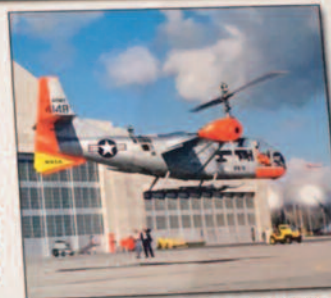
Like a helicopter, tilt-rotor aircraft use their propellers, or proprotors, for vertical lift.
