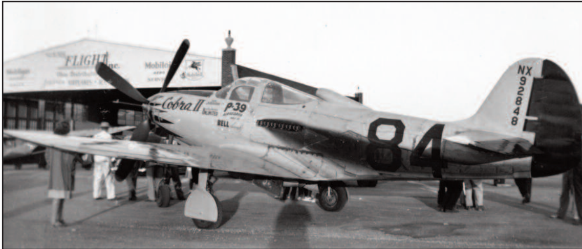
An oil-streaked, race-winning Bell P-39Q Airacobra, NX92848, Tex Johnston's Cobra II. The modified Allison engine's undersized pistons allowed excessive blow-by. (San Diego Air and Space Museum Archives)
