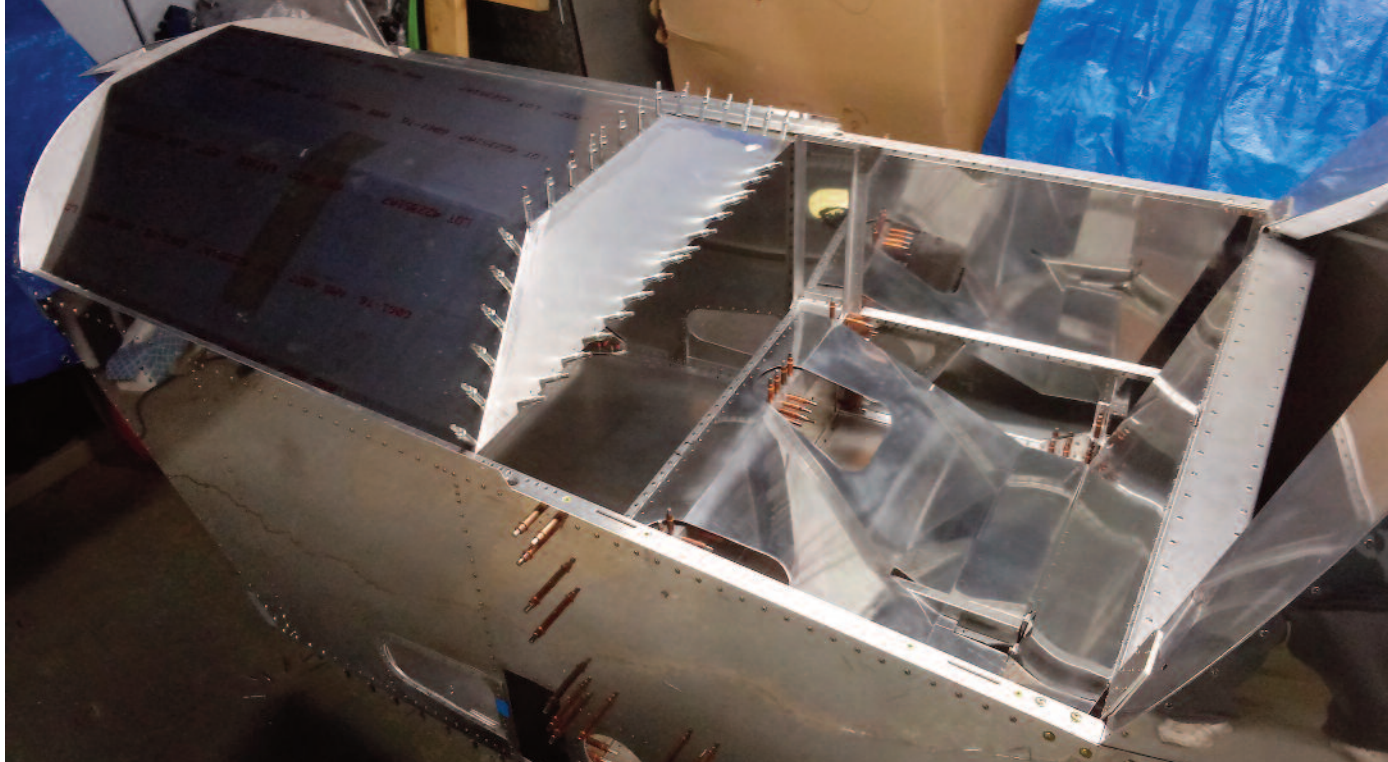
Seat, instrument panel and glareshield in place. Photo Courtesy of Joe Kirik
