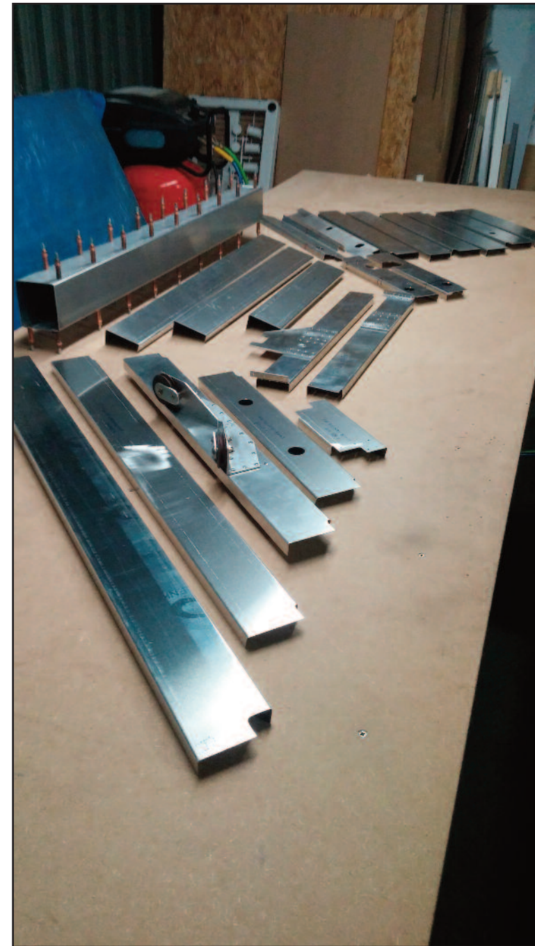
Fuselage tailcone parts made from blank channel stock in my workshop in the back of my hangar at Mettetal. Newer Sonex kits now come with all these parts pre-made!
