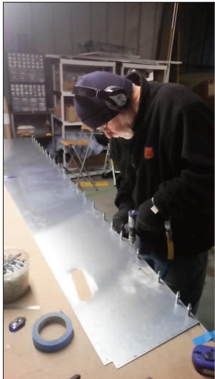
Drilling pilot holes in tailcone longerons using pre-punched holes in the skin as guides.
