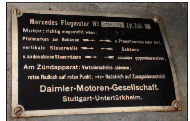
Mercedes engine, used in Fokker D7s and Albatross.
