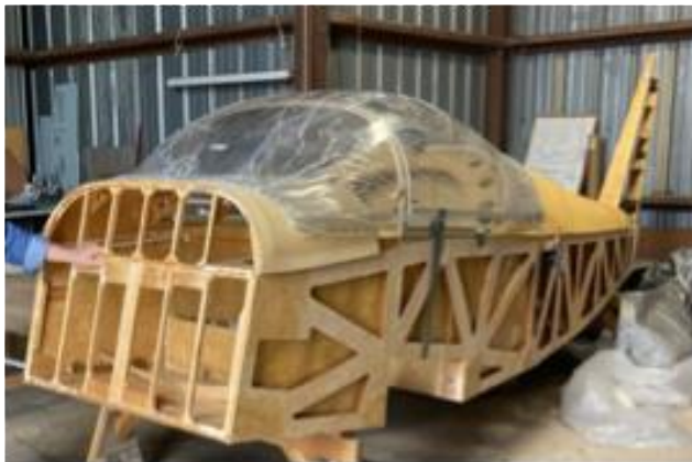
Fuselage framed and ready for controls and finish work
