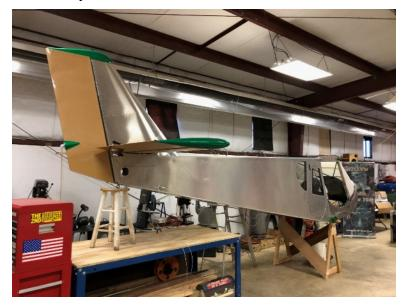
After measuring the length needed for the first wrap of skin down the fuselage side they cut the first piece off a 60 inch wide roll and stretched it out on the aluminum as they began using squeegees to smooth out wrinkles and air pockets beneath the material.
