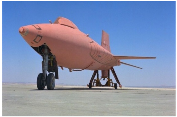
Dryden Flight Research Center ECN-1751 Photographed 1967 X-15 #2 full scale ablation (NASA photo)
