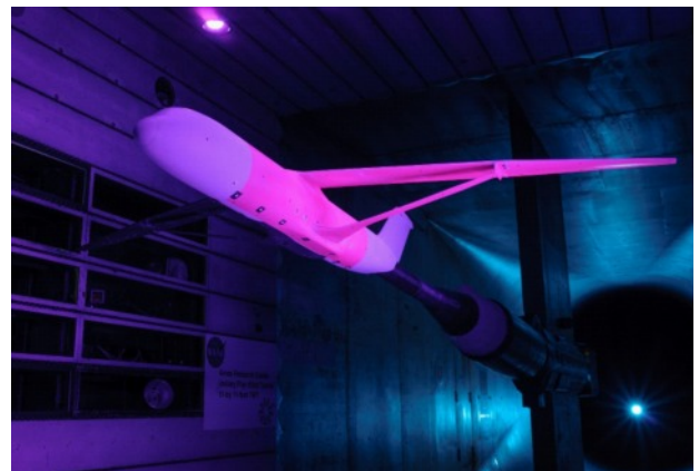
X-66A wind tunnel model with pink PSP (NASA)
