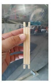
Standoff in use. This allows the top cowl half to stay above engine so I can mark the trim line inside.
