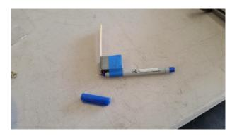
Trim line marking tool in use. This allows me to follow the contour of the top cowl for even spacing of the baffles to the top cowl.
