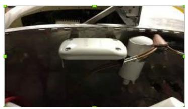
Locating the Receiver/Transmitter (R/T) unit was the next consideration. uAvionix says the R/T is" designed to be mounted in the cockpit, cabin or an avionics bay." But an A&P friend said he'd mounted his R/T in the RV-6 wing, using the inspection plate on the bottom of the wing closest to the fuselage, and it has worked fine.
