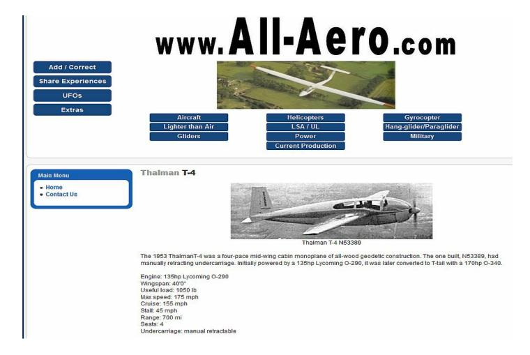
**T-4** 1953 = 4pChwM rg (manual); 135 hp Lycoming O-290; span: 40'0" load: 1050# v: 175/155/45 range: 700. All-wood geodetic construction. [N53389]. Later converted to T-tail with 170 hp O-340. Price FREE.
