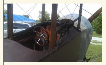
The length is 22'10" with a wingspan of about 25'8". N8184 weighed in at 890 pounds, and will carry a crew weight of 400 pounds with a MAC at 32%. The Sopwith Baby and Sopwith Tabloid are nearly identical, and the Tabloid is typically configured as a side by side 2 seater. Russ's baby is configured as a very wide single seater.
