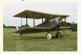
Russ, a retired Air Force flight surgeon has now designed and built two full scale modern reproductions of WWI aircraft. The first, a full-scale Sopwith Camel was featured in the November 2011 Sport Aviation magazine. It is a full scale, welded steel tube and cloth aircraft. Although powered by a 150 HP radial engine and a very large aircraft, it still complies with light sport rules and can be flown as a light sport aircraft.
