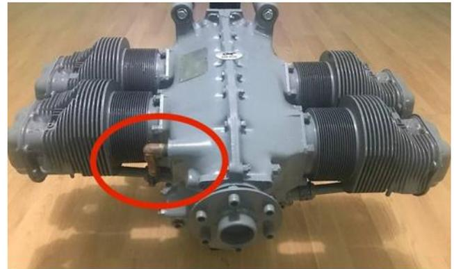
Photo 7: Continental O-200 breather exit. For an aerobatic engine, the brass fitting extends well inside the case whereas the standard brass fitting just threads into the crankcase a short distance. Photo credit: pintrest.com
