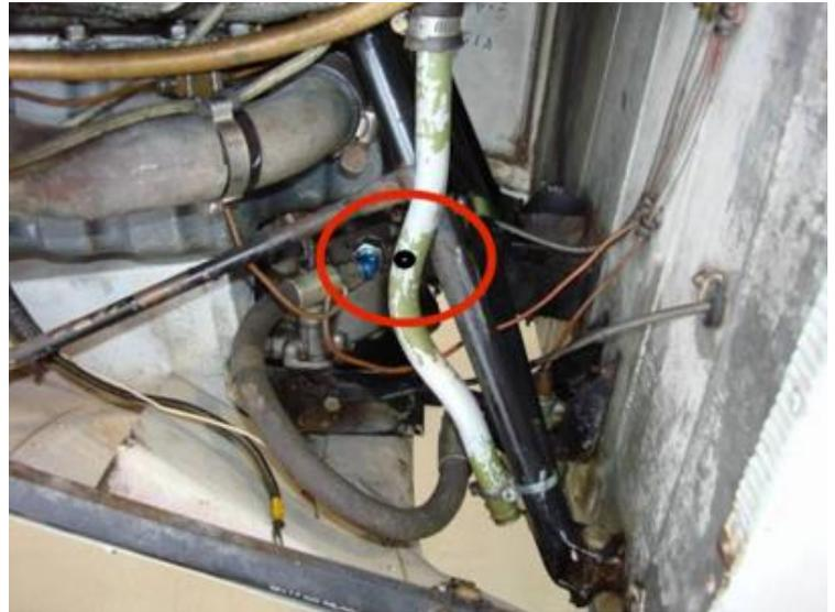
**Photo 2:** Breather line with no ice hole (aka weep hole.) Photo has been edited to show a good location to drill a hole. Photo credit: Supercub.org
