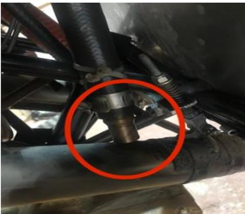
Some experimental builders make their breather tube exit into an empty soup can and occasionally they clean out the can. It is the same idea as the air-oil separator except the captured oil does not drain back into the crankcase.
