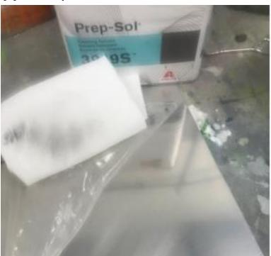
Once the aluminum is clean is needs to be roughened. Not crazy rough, but a sanding with 400 grit or a good scuff with purple Scotch Brite will provide enough "tooth" for the paint to adhere.
