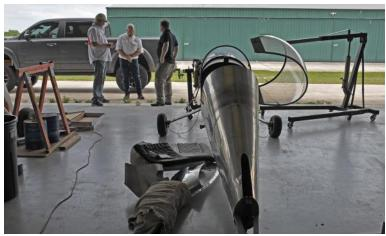
Once the engine was off of the plane, it was mounted to an engine stand for teardown. Being a VW 4-cylinder, it isn't that heavy so manhandling it onto the stand wasn't too difficult.
