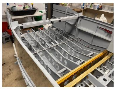
Finally, some gussets were fitted to both sides of the brace to build up the structure for the base of their roll bar. There were plenty of difficult rivets to buck in these tight spaces. Once it was done, I had a nice looking piece which is tying up this section of the plans.
