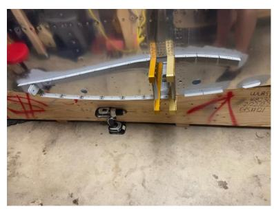
Next, I started building up the brace that also makes up the seat back adjustment rail. Bits of plastic were shaped to make guides for the adjustment arms.
