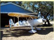
Lyc 0320 (160 hp), newly rebuilt, constant Speed Hartzell Prop, 30 gal fuel tank, new Ceconite fuselage cover, full flying surfaces rejuvenated.
